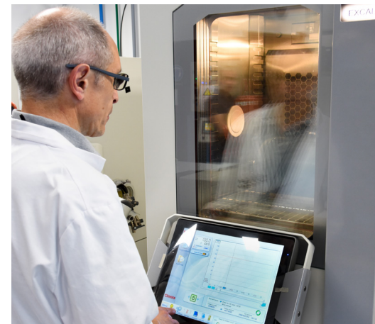
Thermal enclosure for ageing test
